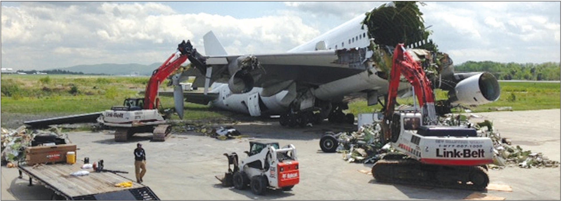
A Boeing 747-200 was parked at Newburgh Stewart International Airport, about 60 miles north of New York City, and Aircraft Demolition and Recycling was called to completely dismantle it.
