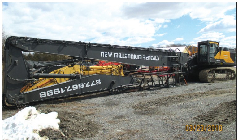
A Volvo 480E HRD with a 93 ft. reach demolition front.
