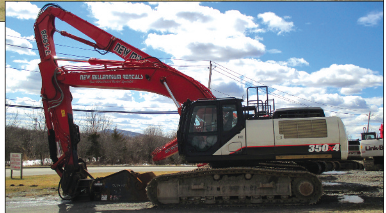
An example from the New Millennium demolition machine fleet, a Link-Belt 350 X4 with a 3rd member mount Genesis GXT series rotating steel shear.
